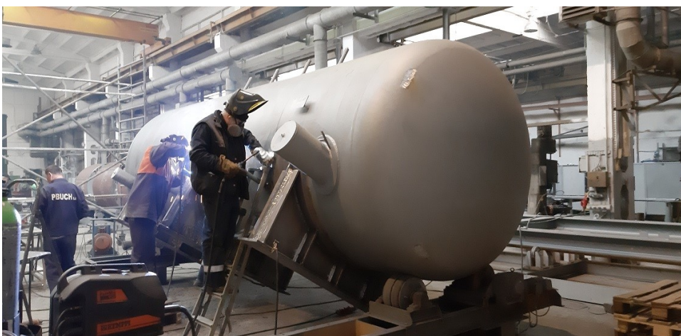
CO2 Separator - hanging construction - calculated with FEA method
