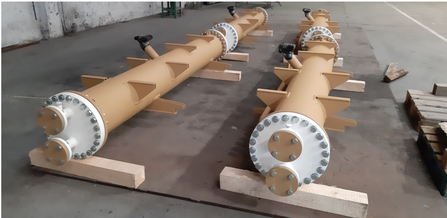
Shell and tube heat exchangers for mining cooling systems
