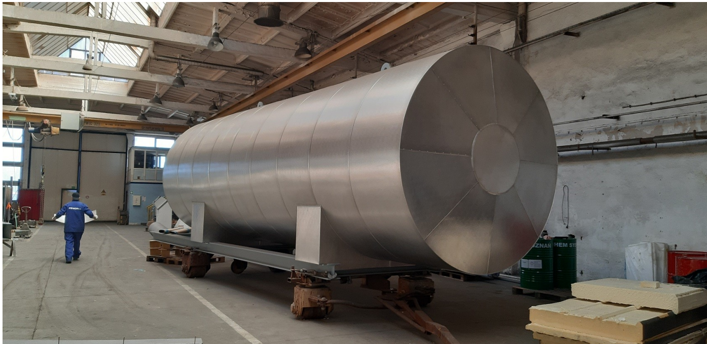
Tank with insulation made of polyurethane foam
