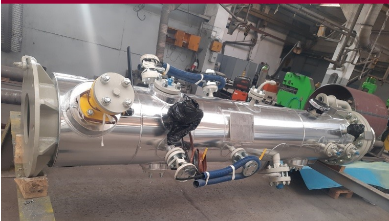
Heat exchanger insulated with mineral wool and a sheet metal mantel
